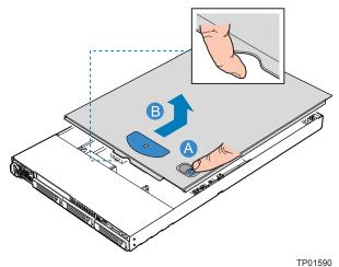
Figure 7. Removing the Chassis Cover
